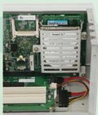
Nuvo-2000 has an ingenious mechanical design which gives consideration to small dimension, superior heat dissipation, flexible wall-mounting, and intuitive pattern of use. Like handling a traditional wall-mount IPC, you can remove the top cover and install add-on cards by loosening a few screws. And its dual SATA ports and dual HDD brackets provide an easy and flexible way to mount your hard drives.
